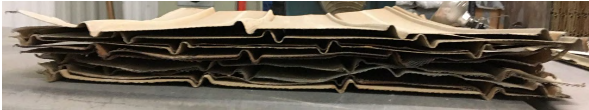
Notches Not Aligned
